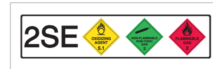
Example of Safety Diamond identification sign
